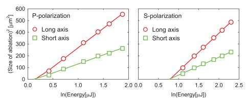
FIG. 2. Examples of the data for the size of the ablation crater squared vs. logarithm of the energy of the ablating laser pulse, for the case of a gold sample illuminated at 45° AOI. The left and right panels show P- and S-polarizations of the incident laser beam, respectively. The two lines of data on each plot correspond to the long and short axes of the elliptical ablation crater. The experimental errors in these data are small compared to the size of the data symbols.
