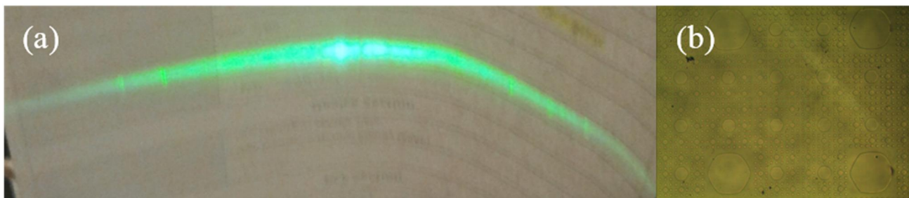
Figure 4 (a) Visual appearance of the beam of generated harmonics incident upon a (curved) white piece of paper. The greenish-blue dominant appearance is consistent with the 4 th harmonic (510 nm), while other harmonics are on the edge or outside of the visible spectrum (2.05 \mu m, 1.02 \mu m, 0.68 \mu m, 0.41 \mu m, 0.34 \mu m). (b) The Sierpinski super-lattice structure of the NPC under a microscope.
